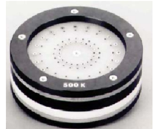
Surface Resistance Calibration Test Fixture
